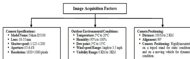
Fig. 1 Camera Setup and Acquisition Factors of TUVD
